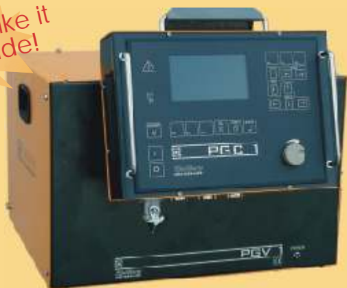
The FlowControl consists of Controller PGC 1 and valve unit PGV 1.
